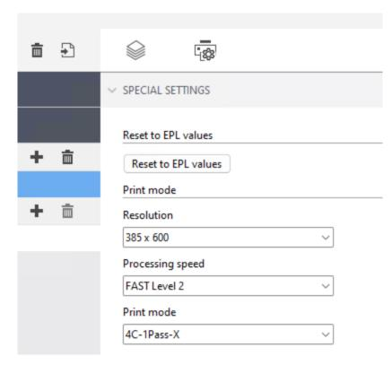
Only resolutions and print modes which are compatible with the color mode of the media profile are available for selection. For example, if the media profile was created for CMYK, only the resolutions and print modes applicable for this color mode are displayed. The Halftone mode should always be set to "Use halftoning from EPL".
